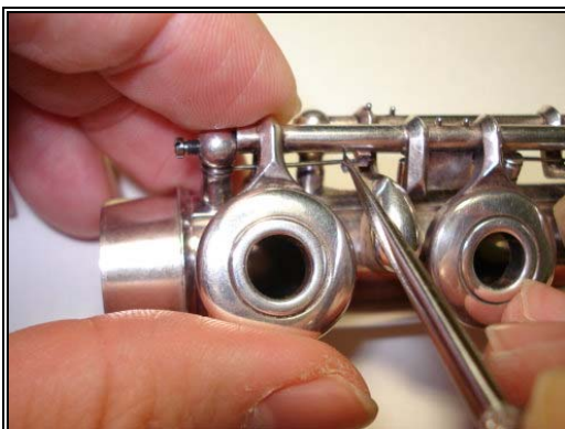
Figure 4.36: Unhooking the D Key Spring
