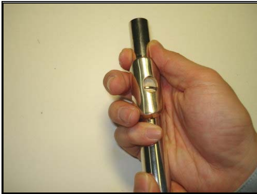
Figure 4.119: Pushing Back the New Cork
