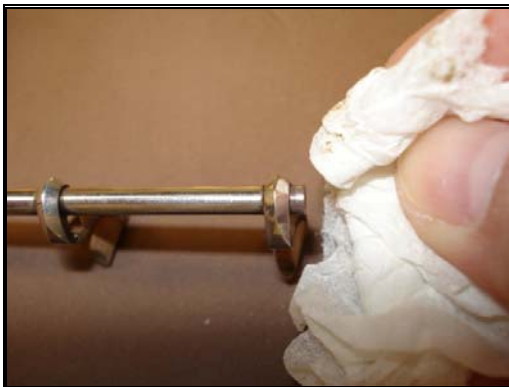
Figure 6.61: Cleaning Both Ends of Trill Key Rod
