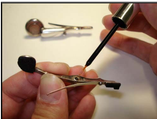
Figure 6.13: Applying a Small Amount of Key Oil
