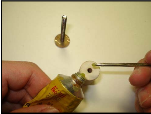
Figure 4.112: Applying Contact Cement Onto One Side
