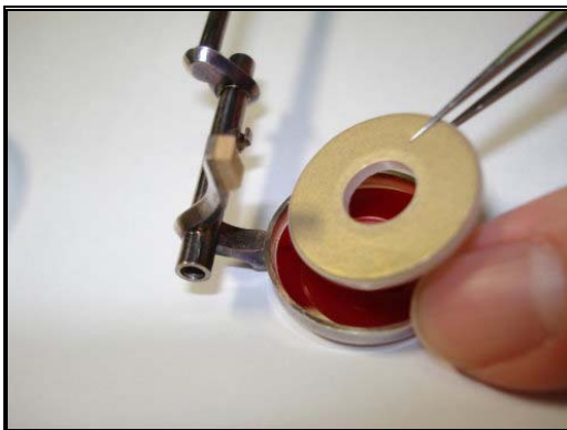
Figure 7.43: Placing the New Gold Pad
