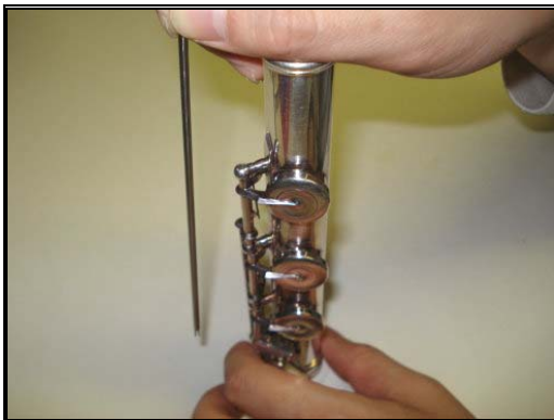
Figure 4.10: Pulling Out the Steel
