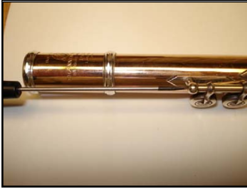
Figure 4.79: Unscrewing the Left-Hand Pivot Screw
