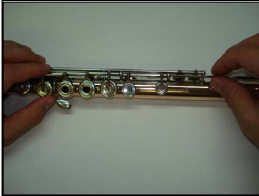
Figure 6.81: Inserting and Tightening Up the Left-Hand Long Screw
