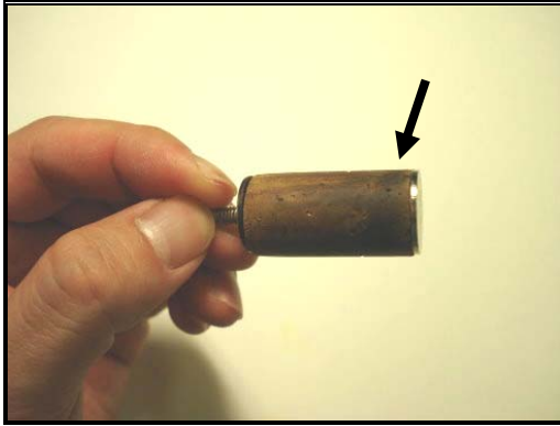
Figure 4.101: Water Gets Into the Bottom of the Cork
