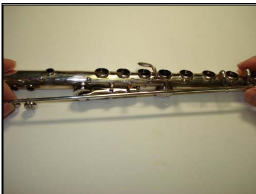
Figure 6.22: Assembling the Trill Key Rod Back
