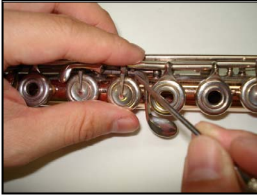
Figure 6.80: Assembling Back G, A, B-Flat and C Keys
