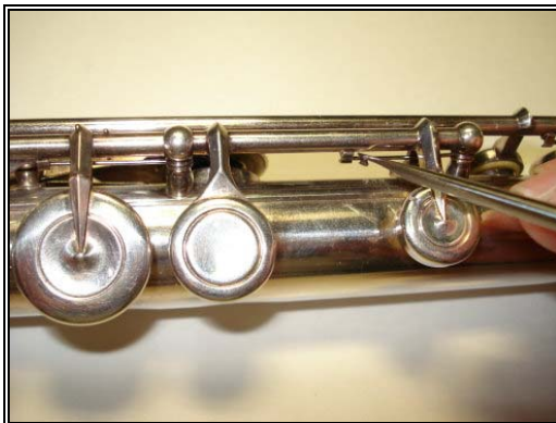
Figure 4.19: Unhooking the B Key Spring
