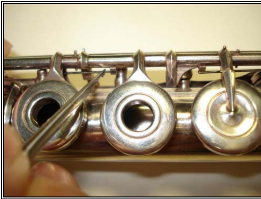
Figure 4.21: Unhooking the A Key Spring
