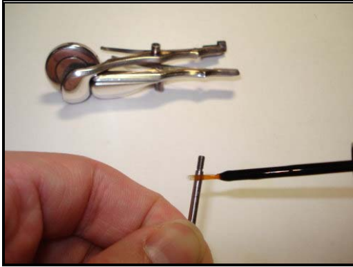
Figure 6.14: Applying Key Oil on the Tip of the Steel
