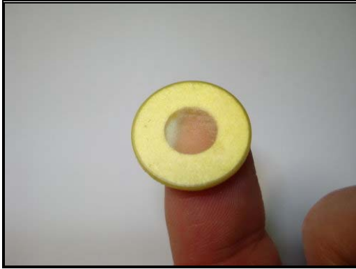
Figure 7.88: Front-View of the Re-Skinned Straubinger Pad
