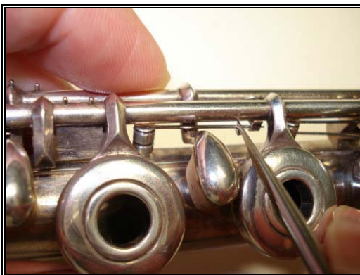
Figure 4.25: Unhooking E Key Spring
