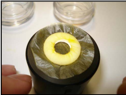
Figure 7.77: Placing the Flattened Skin and Cup onto the Die
