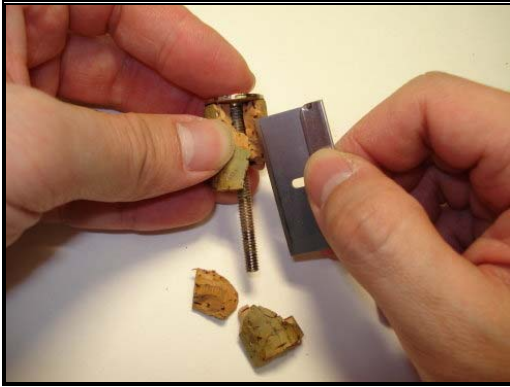
Figure 4.108: Cutting the Cork Vertically
