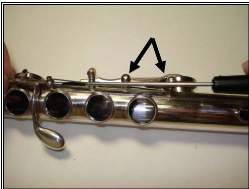
Figure 4.45: Unscrewing the G-Sharp Key
