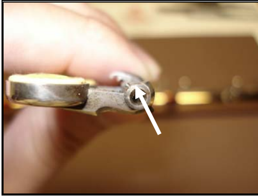
Figure 6.62: Applying Key Oil
