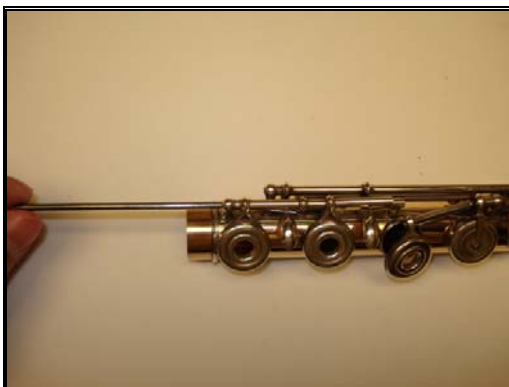
Figure 6.70: Assembling Back F, E and D Keys
