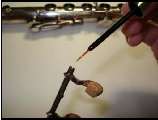
Figure 6.20: Applying Key Oil
