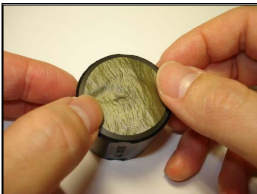
Figure 7.57: Placing the New Fish Skin
