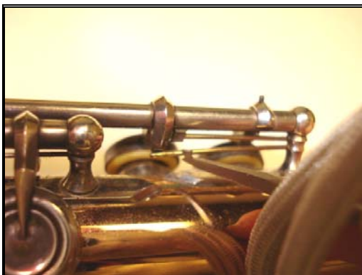
Figure 4.63: Unhooking the Trill Key Springs
