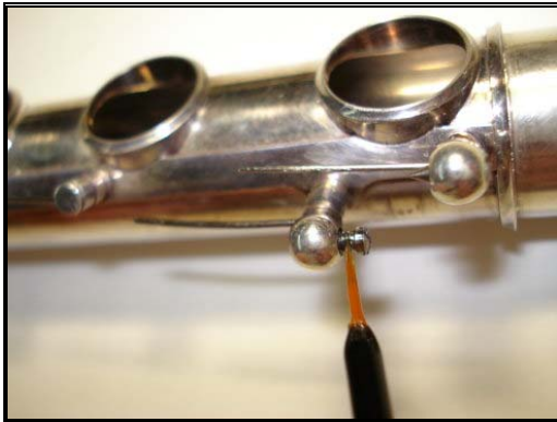
Figure 6.21: Unscrewing the Trill Key Pivot Screws
