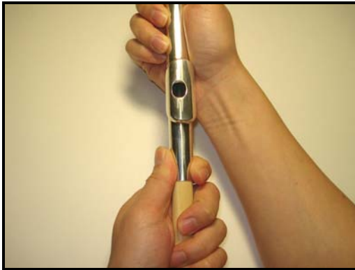
Figure 4.99: Pushing Out the Cork
