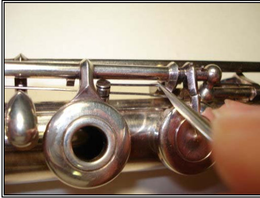
Figure 4.37: Unhooking Upper F Key Spring
