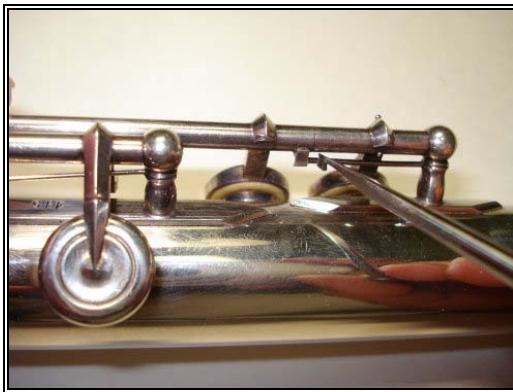
Figure 4.27: Unhooking the Upper Trill Key Spring
