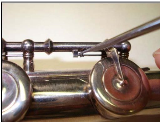
Figure 4.7: Unhooking the Spring of the Low B Key
