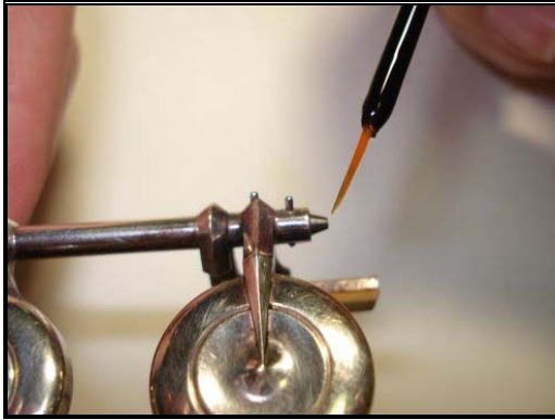
Figure 6.32: Cleaning and Lubricating the Pivot
