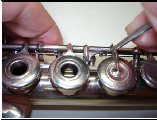
Figure 4.20: Unhooking the B-Flat Key Spring
