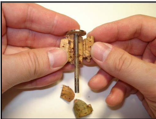
Figure 4.109: Peeling Off the Rest of the Cork
