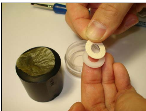
Figure 7.60: Placing Back the Felt Pad
