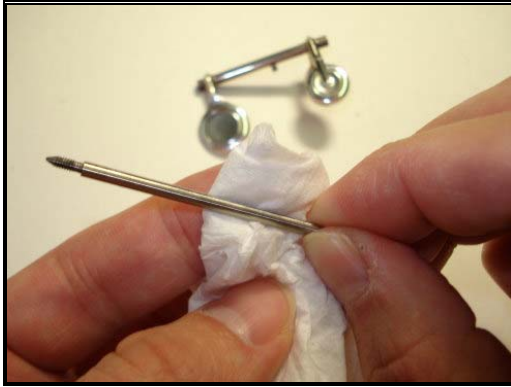
Figure 6.41: Cleaning Off the Oil Residue and Debris
