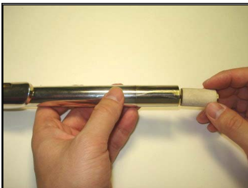
Figure 4.117: Inserting Back the New Cork
