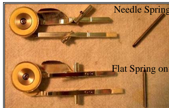
Figure 1.14: The Briccialdi B Flat Thumb Key Photos from Miyazawa Flute Company
