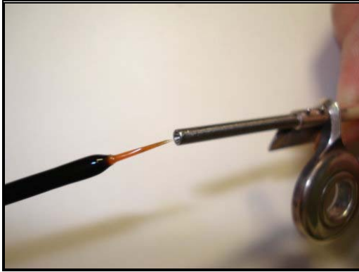
Figure 6.29: Applying Key Oil at the End of the Steel Rod
