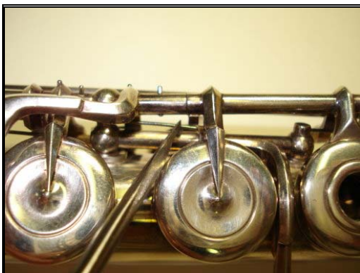
Figure 6.40: Hooking Back the G Key Spring
