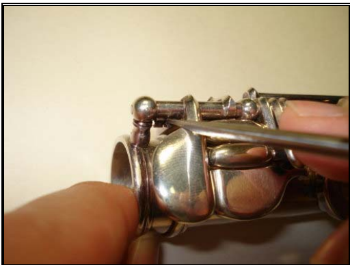
Figure 4.4: Pushing the Spring Off the Spring Catch
