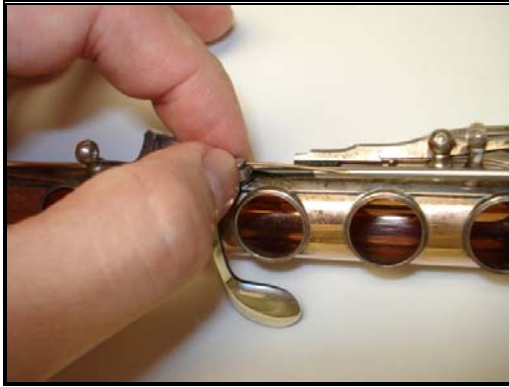
Figure 4.85: Unscrewing the G-Sharp Key
