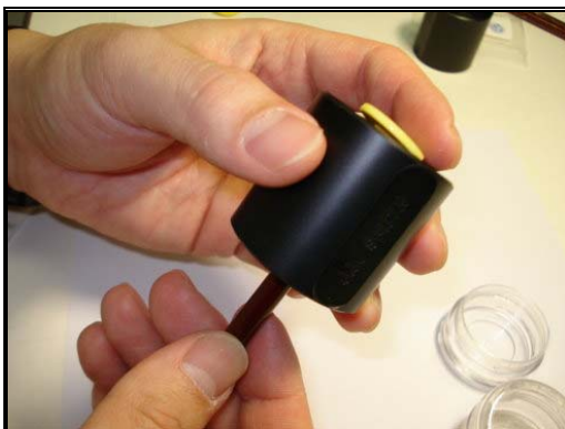
Figure 7.72: Removing the Pad
