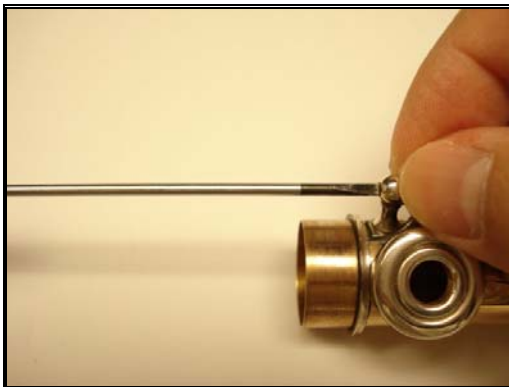
Figure 4.72: Unscrewing the Right Hand Key Steel
