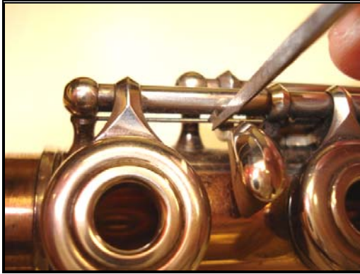
Figure 4.62: Unhooking the D Key Spring
