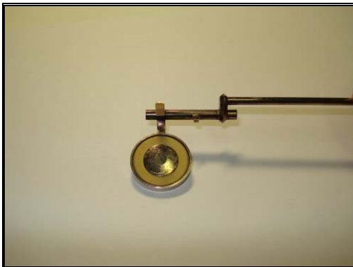
Figure 7.47: Completed New Jim Schmidt Gold Pad Installation
