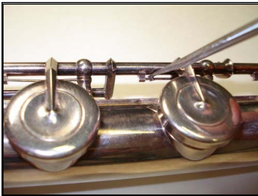
Figure 4.6: Unhooking the Spring of the C-Key
