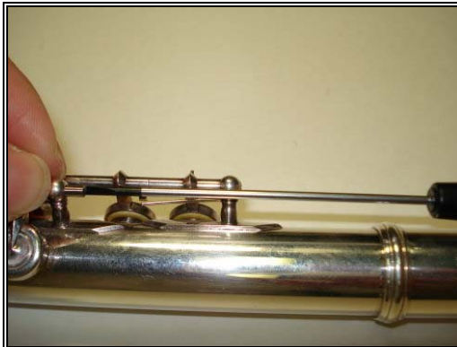
Figure 4.30: Unscrewing the Steel
