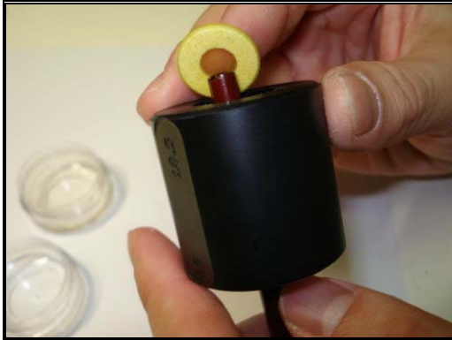
Figure 7.86: Removing the Pad
