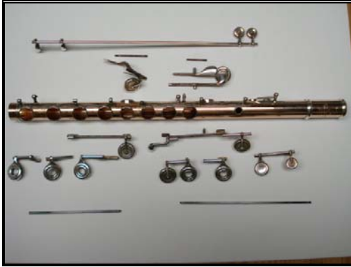
Figure 4.94: All the Disassembled Components of the Brögger mechanism
