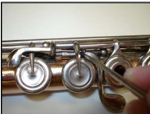
Figure 4.69: Unhooking the G Key Spring
