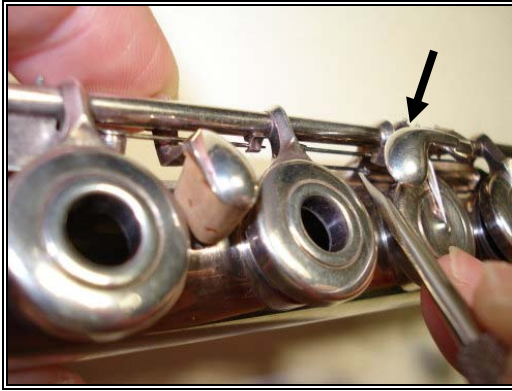
Figure 4.23: Unhooking the F-Sharp Key Spring
