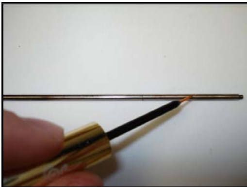
Figure 6.69: Applying Key Oil onto Tip of the Screw
