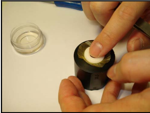
Figure 7.62: Press the Pad Cup Support And Synthetic Felt
