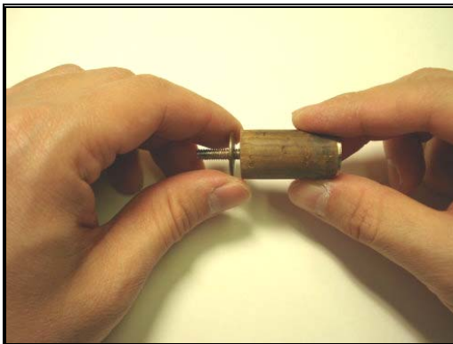
Figure 4.102: Unscrewing the Upper Metal Disc
