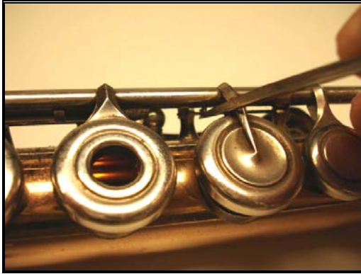
Figure 4.58: Unhooking the B-Flat Key Spring
