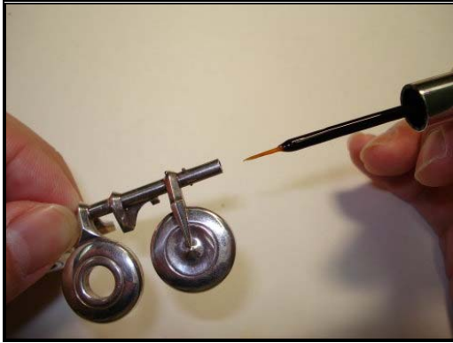
Figure 6.38: Applying Key Oil
