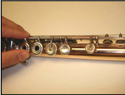
Figure 4.68: Pulling Out the Left-Hand Screw
