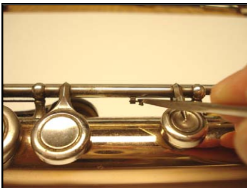
Figure 4.57: Unhooking the B Key Spring
