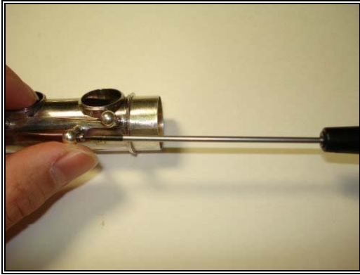
Figure 4.43: Right Trill Key Pivot Screw
