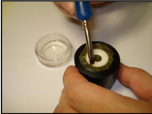
Figure 7.65: Applying the Mucilage
