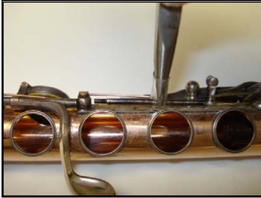
Figure 4.88: Pulling Out the Steel Completely
