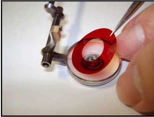
Figure 7.42: Placing the Plastic Shim
