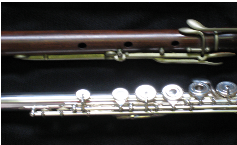
Figure 1: Comparison of Pre-Boehm and Modern Flute Mechanisms
