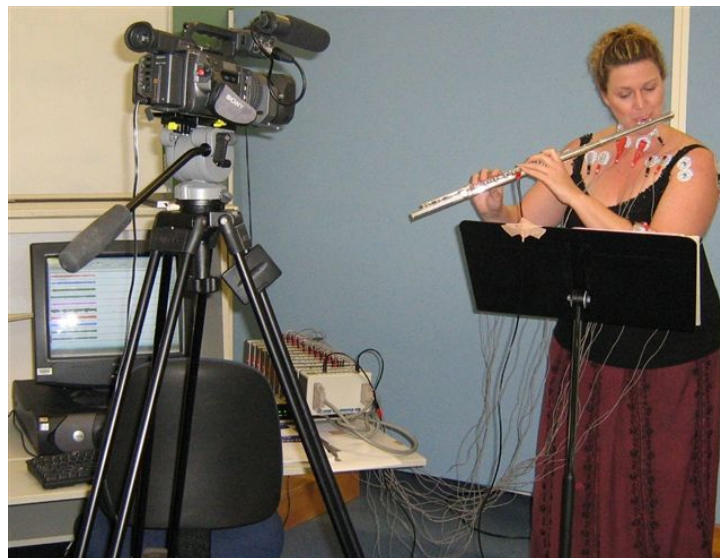
Figure 7: Full EMG Set-Up
